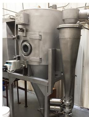
Figure 4: Encapsulation via Spray Drying (pilot scale)
